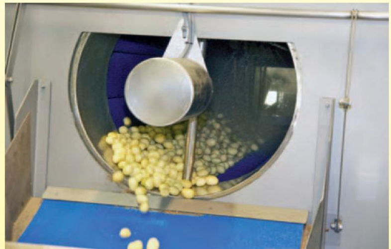
Fully open side panel gives EASY ACCESS FOR BRUSH ROLLER REMOVAL
